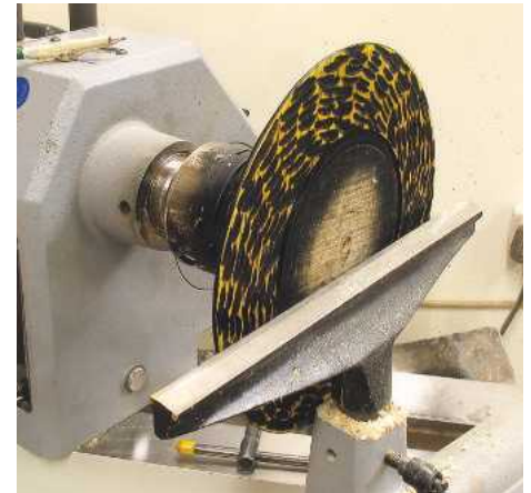
▲ Pic.21 To give easy access to the bowl centre Les has swivelled the head on the lathe. If you intend to do a lot of bowl and box work it's worth taking a look at a lathe with this facility
